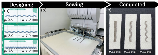
FIGURE 3. Procedure for fabrication of embroidery bend sensors.
