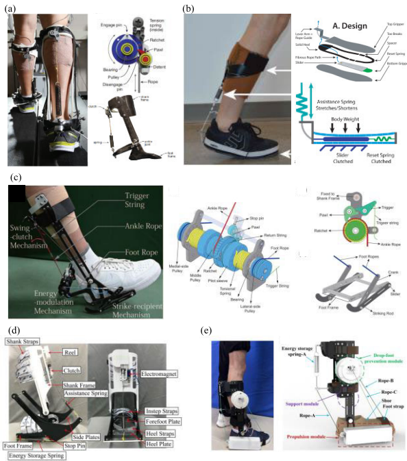
FIGURE 3. Ankle-foot (quasi-)passive exoskeletons and their specific structures. (a) ankle passive exoskeleton and its clutchspring mechanism [10] (b) ankle passive exoskeleton [18], (c) anklefoot passive exoskeleton and its mechanical controller [16] (d) quasipassive ankle-foot exoskeleton [17] (e) ankle-foot exoskeleton with propulsion module and drop-foot prevention module [19].
