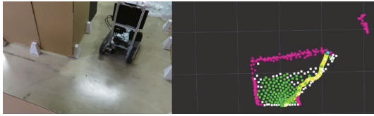
FIGURE 16. The state of movement (Traversability). The left side shows the robot in motion, and the right side shows the learning process in GNG-DT. The green nodes represent traversable node, the black nodes represent untraversable, the white nodes are candidate subgoal nodes, and the red nodes are obstacles. The green circle is the current node and the light blue circle is the destination node, and the yellow line is the result of local planning connecting these two points.
