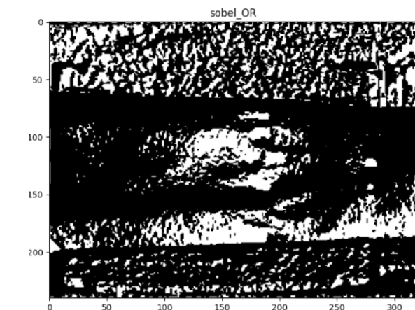
FIGURE 11. Combined Sobel gradient image, highlighting both horizontal and vertical edges.
