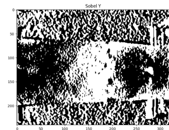
FIGURE 10. Sobel Y gradient result, highlighting vertical edge detection.
