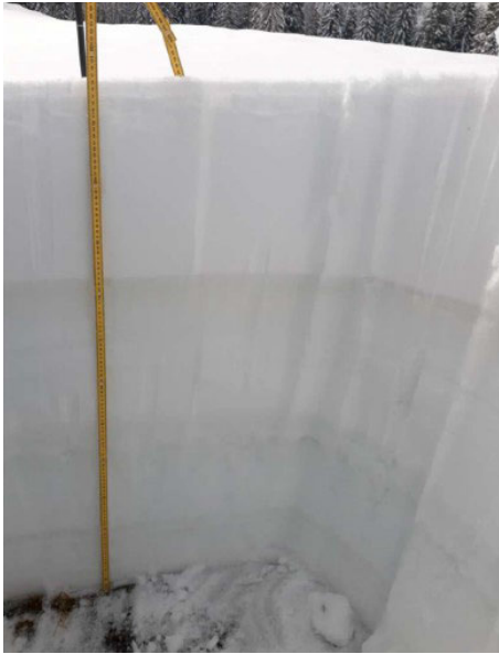
FIGURE 7. The snowpack stratification shows a clear visual distinction between the new snow deposited in the last 72 hours (surface layer H 116-82 cm, white color) and the old snow present before the recent snowfalls ( H 82-0 cm, darker color).
