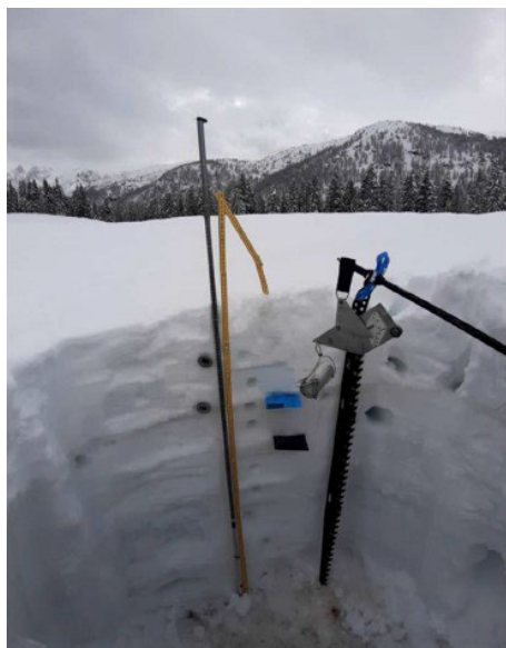
FIGURE 6. The instrumentation used for vertical analysis of the snowpack (snow profile).
