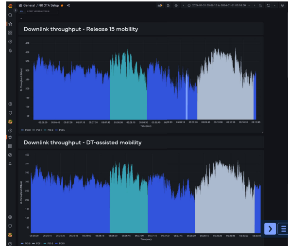
FIGURE 16. Throughput and serving cell PCI over time for baseline Rel15 mobility and DTAM runs obtained from Qualcomm Edgewise PM dashboard.
