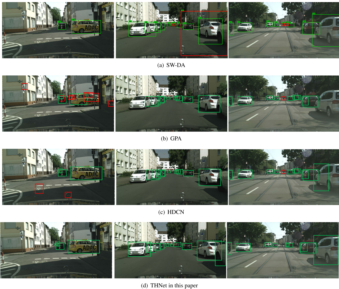
FIGURE 7. Detecting results of different methods on the synthetic-to-real task. Note that green rectangular boxes indicate rightly detected targets, while red ones indicate incorrectly detected targets.
