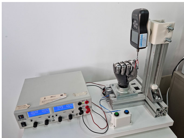
FIGURE 5. Experimental testbed. On the left, the power supply is visible; on the right, the prosthetic hand is mounted on the test rig, with the index finger hooked to the measuring tool in the top-right corner. At the front, the two-button console used to issue the opening and closing signals for the finger is also shown.
