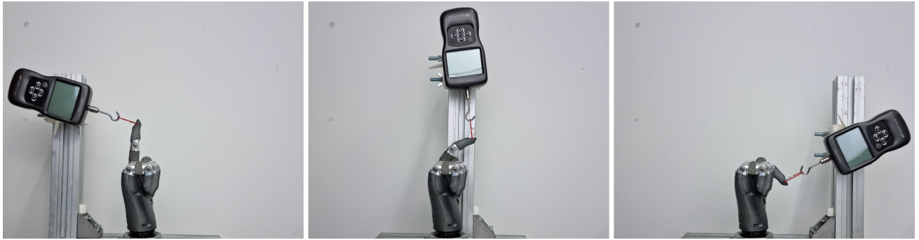
FIGURE 7. Demonstrative sequence of traction tests for finger force measurement.
