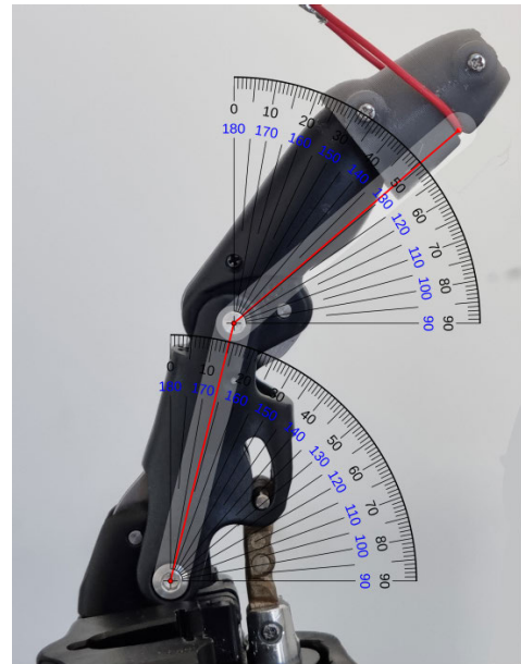
FIGURE 9. Extraction of the rotation angles of the proximal and distal phalanges from the high-resolution image of the finger.
