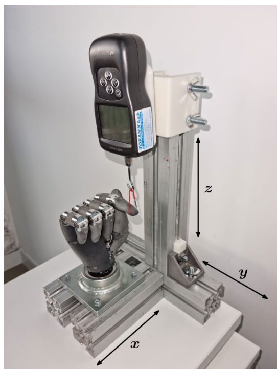
FIGURE 6. Detailed view of the fixture system and measuring head. The supporting plate, which incorporates the quick-disconnect wrist (QDW) attachment for the prosthetic hand, can be moved along the x -axis. The vertical upright can slide along the y -axis, and the 3D-printed white block can be adjusted along the z -axis. This enables the precise repositioning of the measuring tool within the y - z plane relative to the finger.
