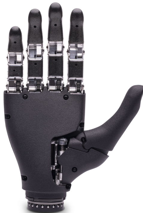
FIGURE 1. Adam's Hand: the underactuated prosthesis proposed by BionIT Labs [15].
