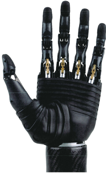
FIGURE 3. Bebionic v2: the fully-actuated prosthesis proposed by Steeper [20].
