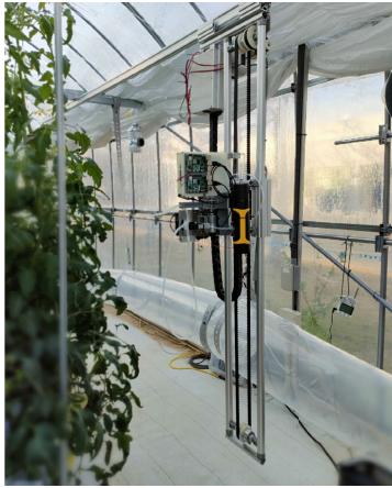
FIGURE 1. A suspended pollination robot with a flexible multi-degrees-of-freedom manipulator and a blower.
