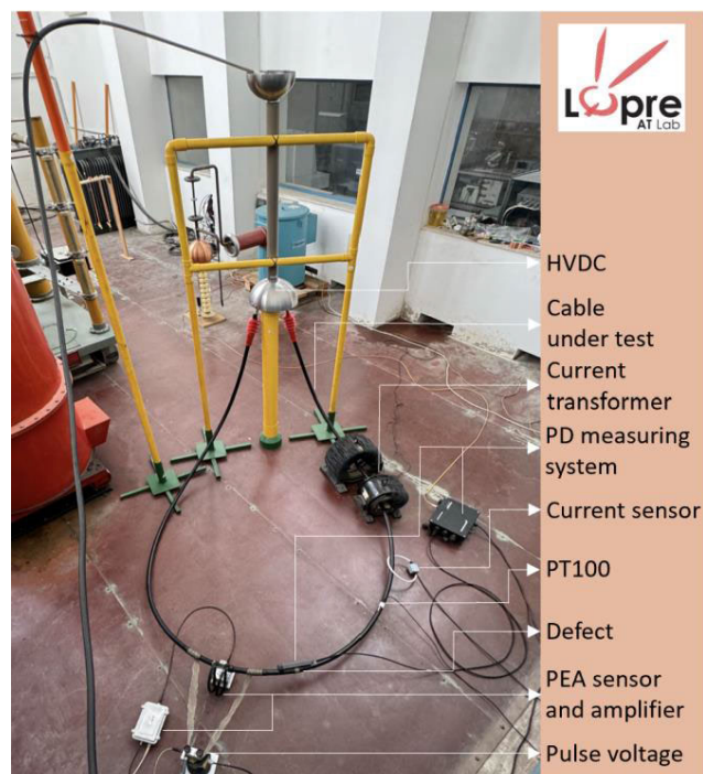
FIGURE 5. The arranged measurement setup for the simultaneous detection of space charge and PD in a DC model cable under operating conditions.
