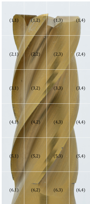
FIGURE 9. Fragmentation of an image of an integral spiral endmill into 24 parts.
