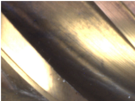
FIGURE 2. Light reflection on TiN coated endmill. The light is reflected back most strongly at the edges of the cutter, whereas shadowing occurs in the inner rake space.
