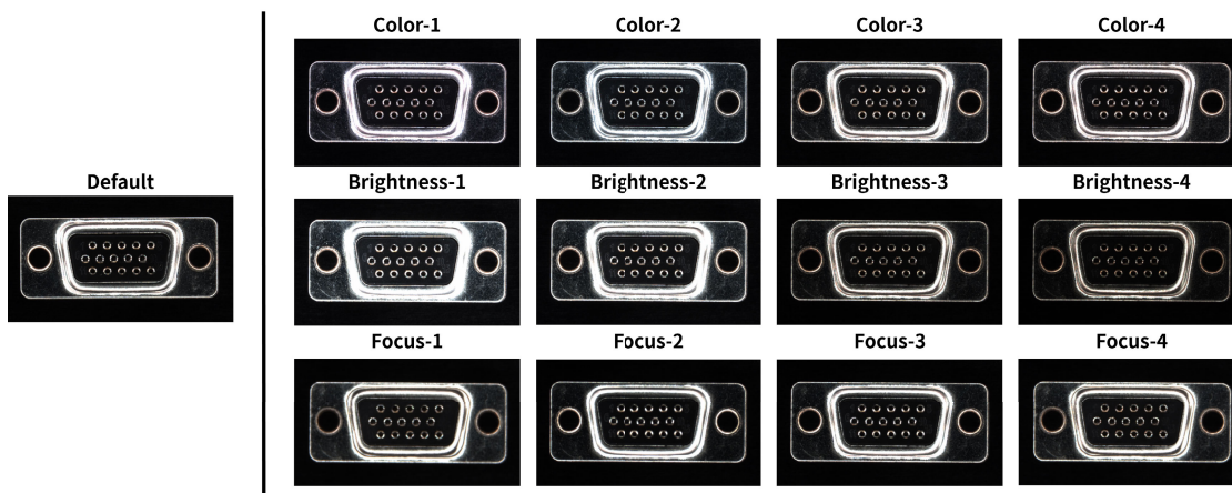
FIGURE 5. Representative examples of each 13 different environments from OK class. Based on the Default environment, there are three environmental factors (Color, Brightness, and Focus), each with four configuration settings depending on its intensity.
