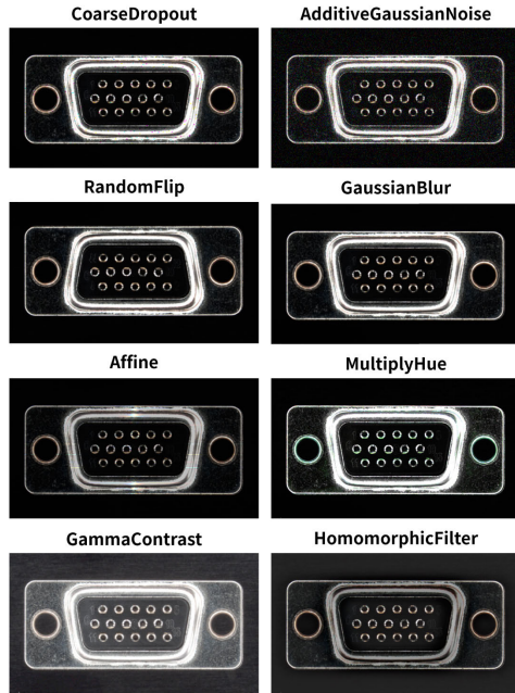
FIGURE 6. Representative examples of each type of image transformation to be used for creating augmented domains.
