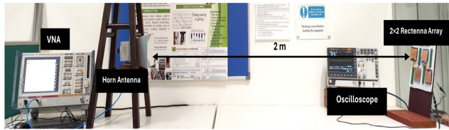
FIGURE 13. Experimental setup for the proposed meta-patch rectenna array.
