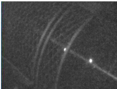
FIGURE 4. Visual corona at 45kV for ambient temperature measurement.
