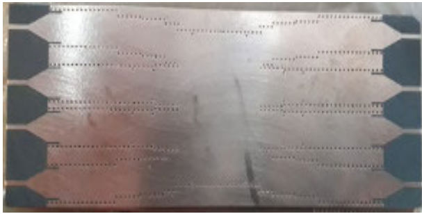
FIGURE 8. Eight-port directional coupler manufactured in SIW technology.
