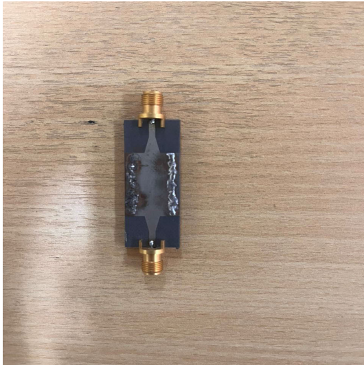
FIGURE 24. SIW microstrip transition WR-51.
