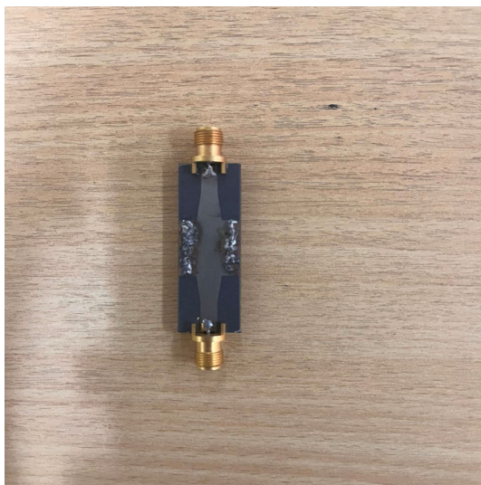
FIGURE 22. SIW microstrip transition WR-62.
