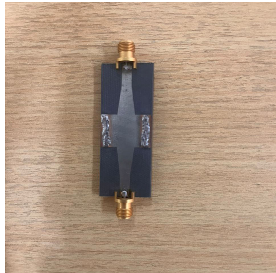
FIGURE 20. SIW microstrip transition WR-75.
