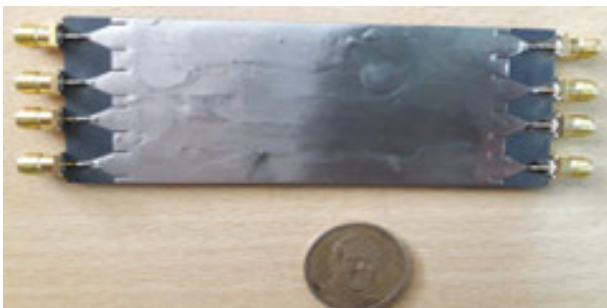
FIGURE 9. Eight-port directional coupler manufactured in SIW technology with SMA connectors.
