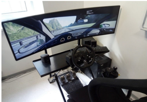
FIGURE 2. The used simulator platform.
