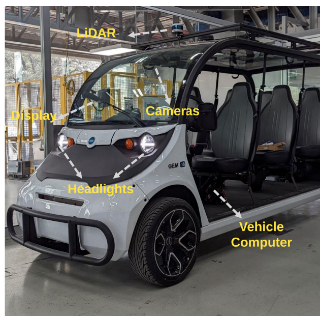
FIGURE 15. On-field experimental autonomous vehicle platform to evaluate HMI elements at Tecnológico de Monterrey.
