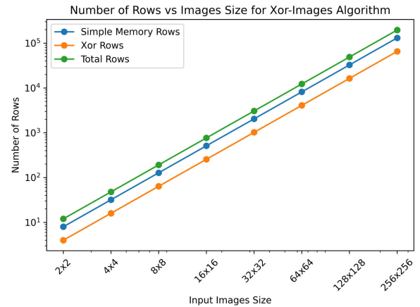
FIGURE 5. Number of "Simple memory" and "Xor" rows for each Octantis' synthesis run with a different images size.
