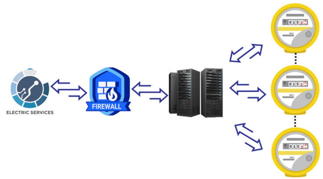
FIGURE 2. AMI network in smart grid [2].
