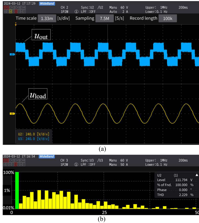
FIGURE 25. (a) Waveforms of the inverter and load voltages and (b) results of harmonic analysis of the load voltage (values of harmonics are related to the fundamental harmonic and the result is presented in logarithmic scale). RMS value of the load voltage is 110 V and its THD is 2.229%.
