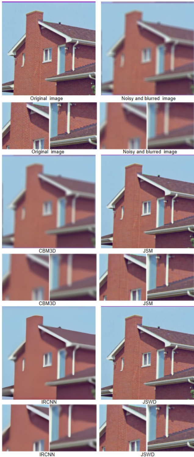
FIGURE 5. The sequence from left to right displays the original, unaltered image, succeeded by the image that has been corrupted by noise and subjected to mean blurring. Subsequently, the deblurring results of the algorithms CBM3D, JSM, IRCNN, and JSWD are exhibited on the test image 'House'. The subsequent pair of diminutive images provide a detailed, localized view for an in-depth analysis.
