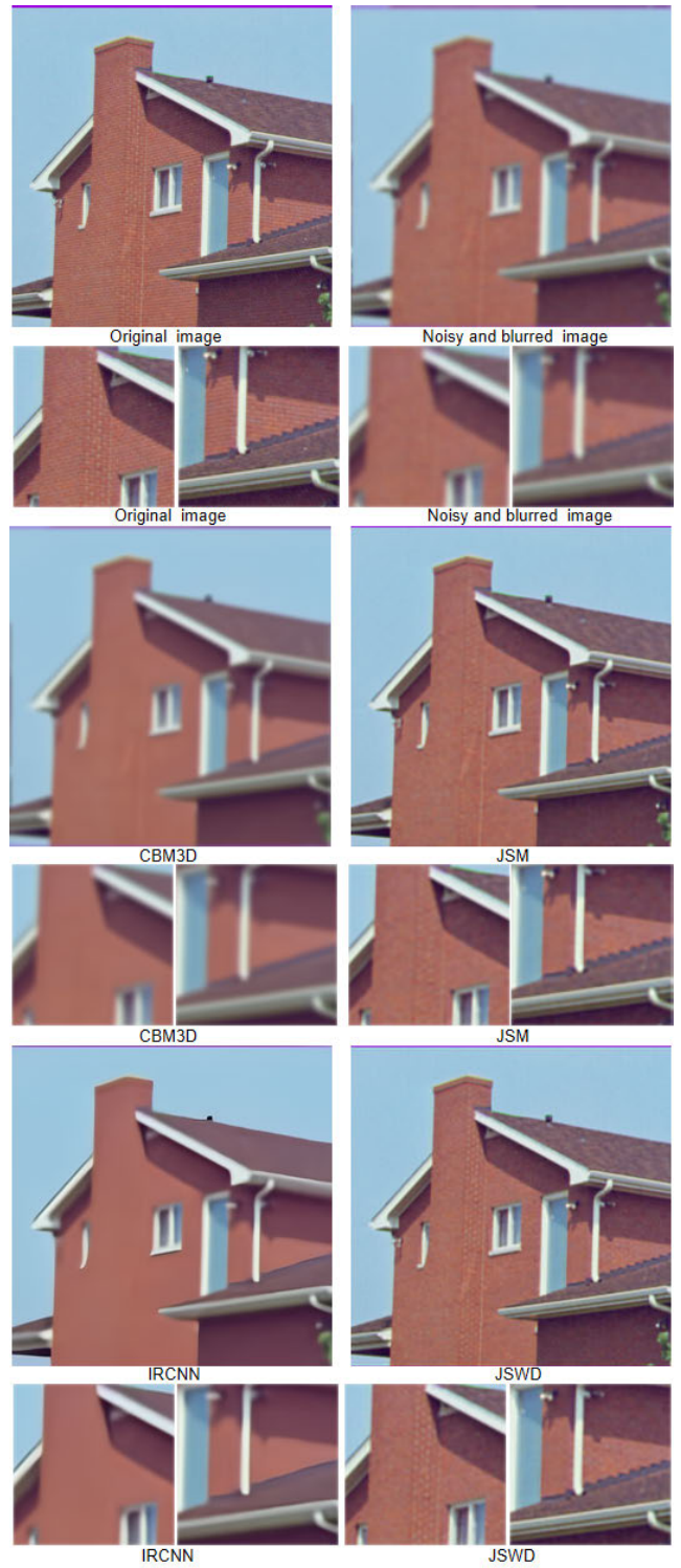
FIGURE 6. The sequence from left to right displays the original, unaltered image, succeeded by a version marred by noise and Gaussian blurring. Subsequently, the deblurring outcomes of the CBM3D, JSM, IRCNN, and JSWD algorithms are delineated on the exemplar image 'House'. The subsequent pair of diminutive images provides a localized view for detailed scrutiny.
