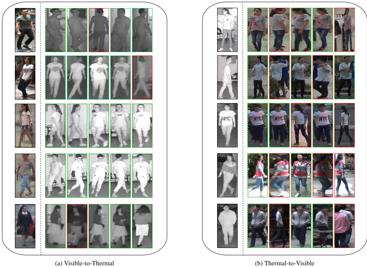
FIGURE 3. Image similarity check is done by randomly sampling ten identities from the gallery and trying to match images in two settings: (a) Visible-to-Thermal, (b) Thermal-to-Visible. Green boxes indicate a correct match, and red boxes indicate a wrong match.
