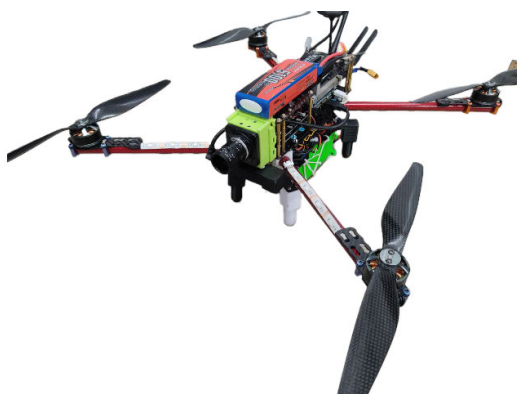
FIGURE 5. Autonomous drone implementation for facial recognition and tracking.
