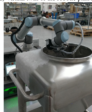
(b) Robotic platform scanning the inner surface of the bin.
