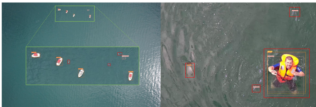
FIGURE 2. Some failure examples with FPN. (The red boxes in left indicate missed detections, while it represents false positives in right.)
