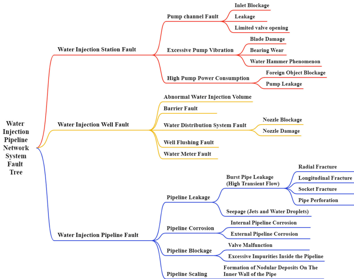
FIGURE 2. Fault tree of water injection system.
