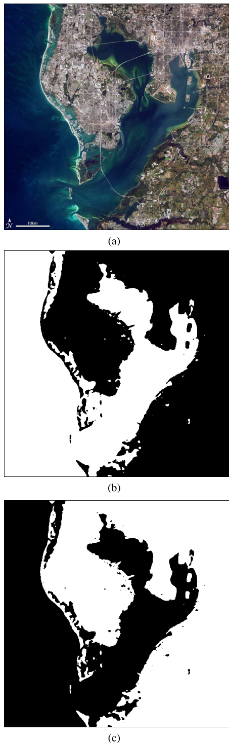
FIGURE 13. (a) Satellite image of Tampa Bay, FL. (downloaded from NASA Earth Observatory) (b) Processed binary image from Fig. 13a for the USV and UUV; (c) Processed binary image for UGV, which is an inverse of Fig. 13b.
