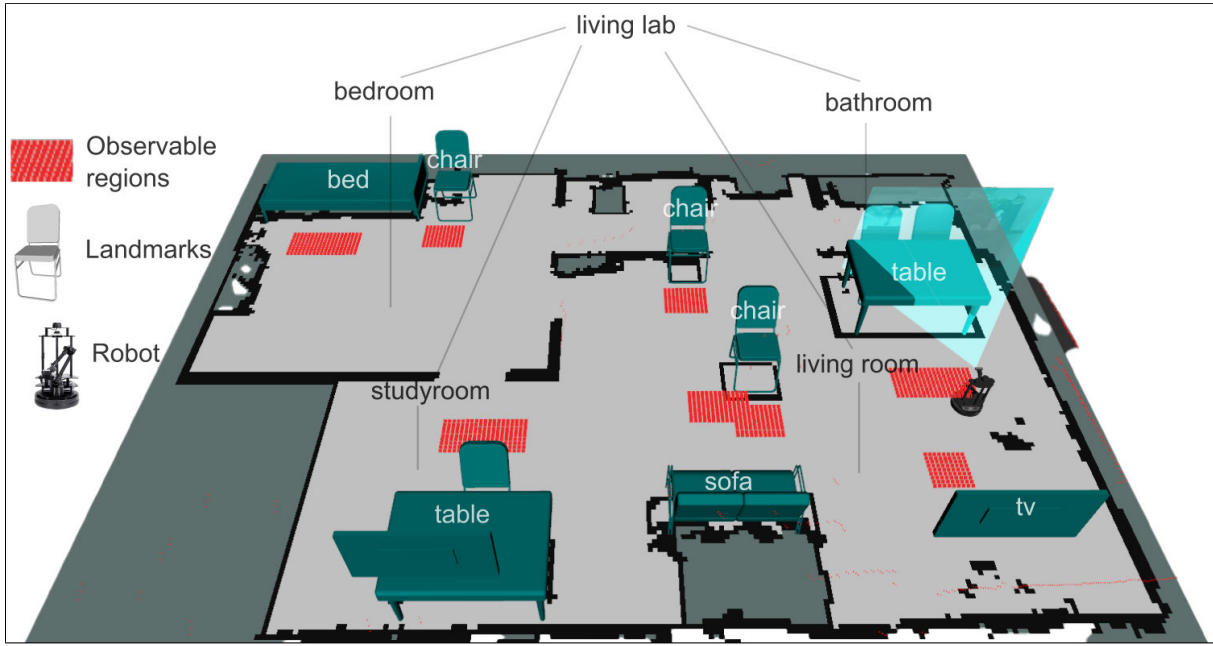
FIGURE 2. Robot navigation in the semantic map. First Layer: metric grid map with obstacle information as occupied cells. Second layer: landmarks shown by CAD models. Third Layer: observable regions shown by red grids.
