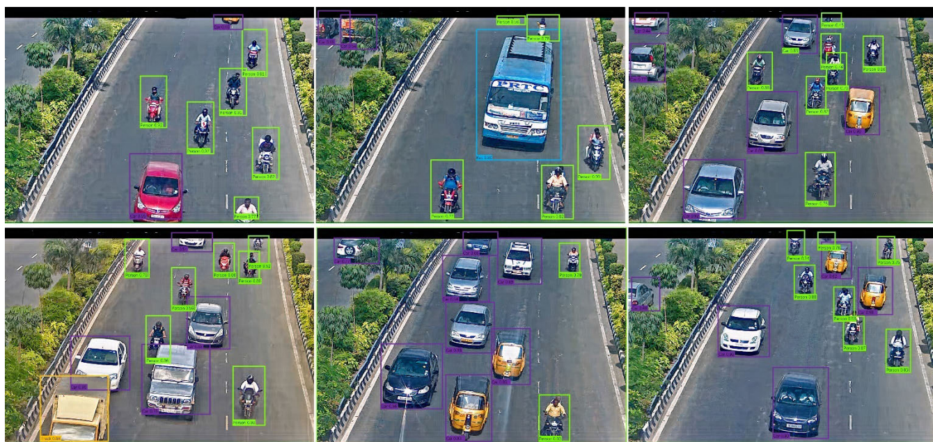
FIGURE 11. Some result images on the IITM-hetra dataset are shown in figure. Augmented by our proposed SSIGAN model and then detected by GCAFormer.
