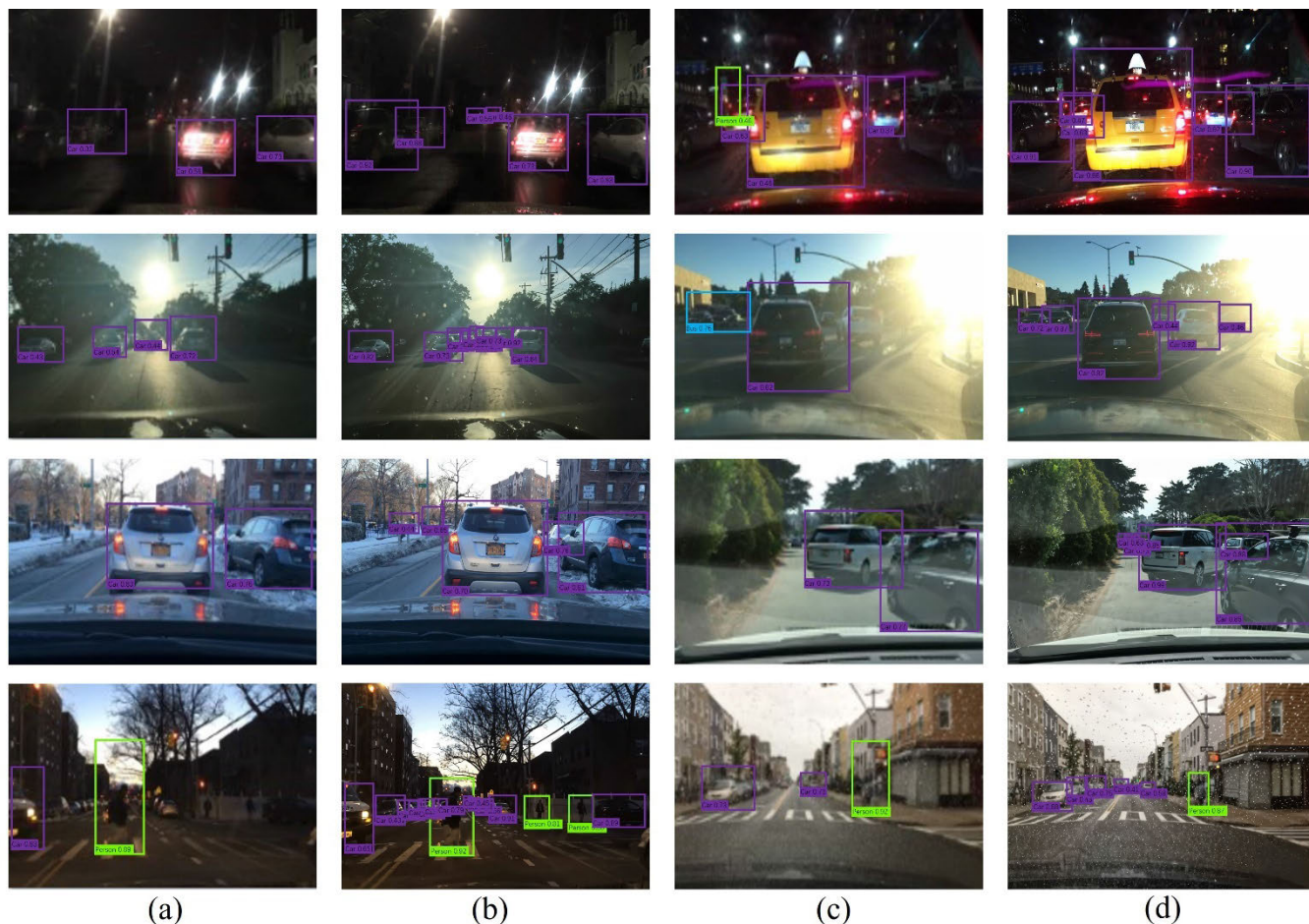
FIGURE 13. (a) and (c) show the resultant images of GCAFormer model detection at low resolution. (b) and (d) show the SR images enhanced by the SSIGAN model and then detected by the GCAFormer model.
