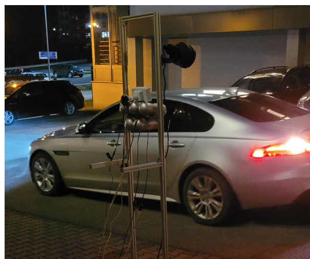
FIGURE 10. The proposed sensing system capturing images of vehicles during the verification at the UNIZA (University of Žilina) parking lot.
