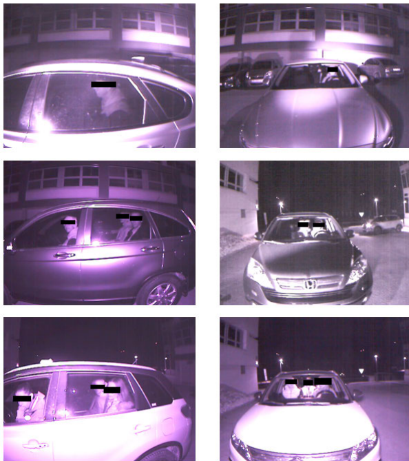
FIGURE 11. Various types of images captured by a camera with an NIR filter. Top row: Jaguar XF, middle: Honda CRV, bottom: Suzuki Vitara.
