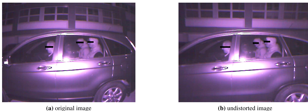
FIGURE 9. Comparison between the original image (left) and the image after distortion removal (right) obtained from a camera equipped with a NIR filter.
