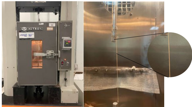
FIGURE 3. Experimental setup for isometric and eccentric contractions. Instron environmental chamber with support fixed to TCP sample at the lower end, and to the Instron load cell at the top end (left); b) Inside view of environmental chamber during actuation with TCP sample ends fixed (right).
