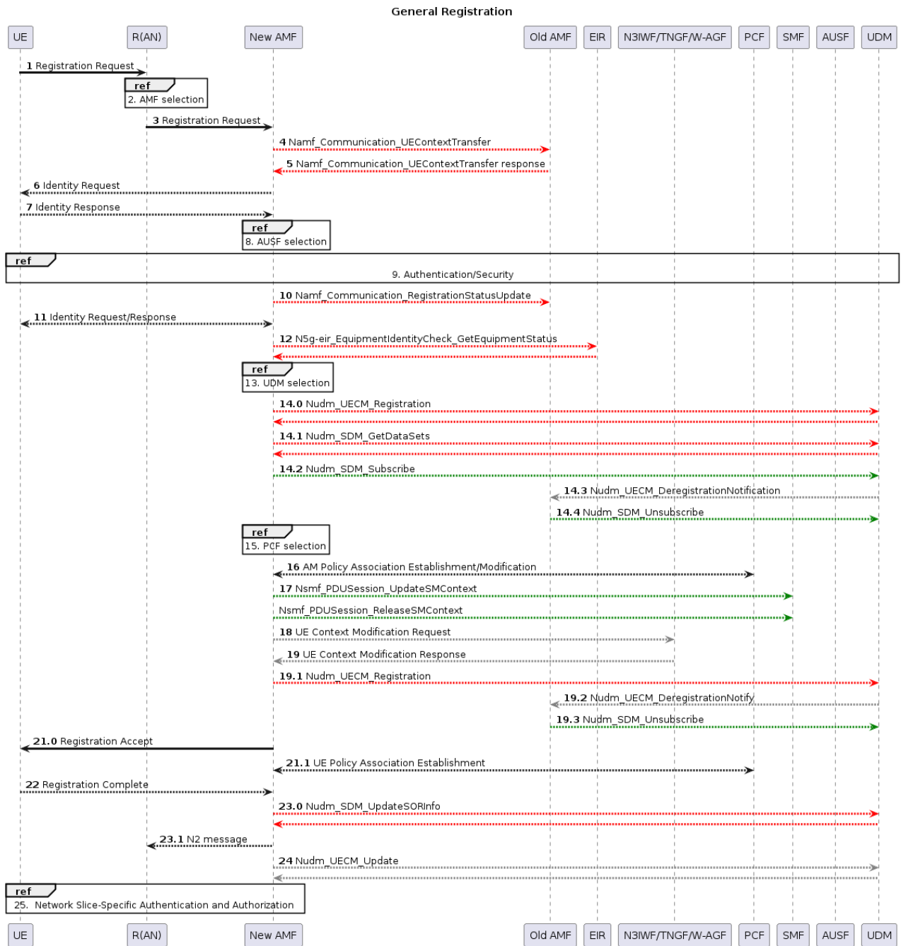
FIGURE 14. Open5GS: UE Registration procedure.
