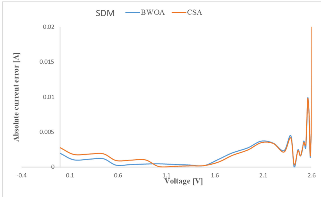
FIGURE 14. Absolute current errors calculated using BWOA and CSA algorithms for the SDM model.
