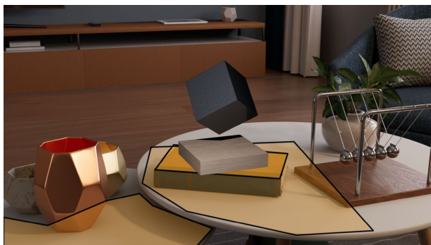
FIGURE 6. AR content (cube with a wooden base) placed on planes tracked in the environment (orange surfaces).
