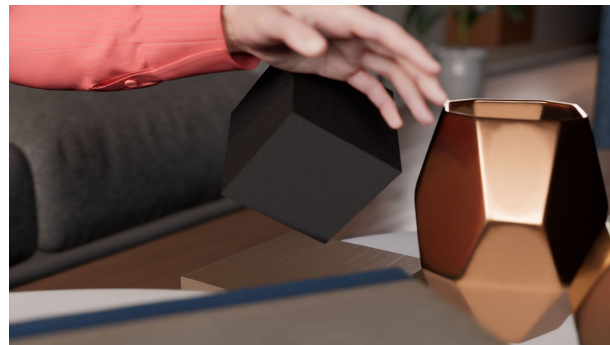
FIGURE 19. AR content with occlusion applied. It is now occluded by real-world objects in front (the book and the hand), giving a proper sense of depth.
