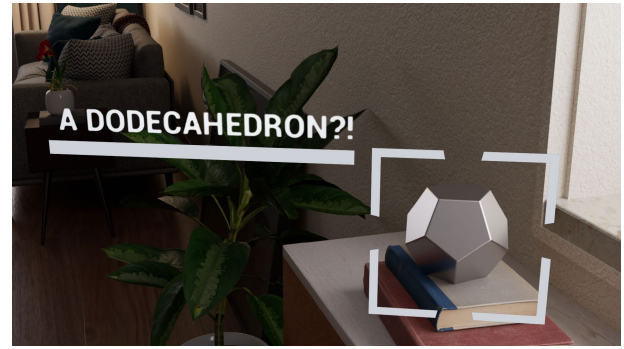
FIGURE 11. AR content (text and target marker) placed with object tracking.
