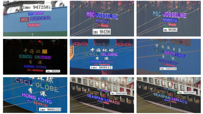
FIGURE 15. Text recognition of ship IMO region by ABINet.
