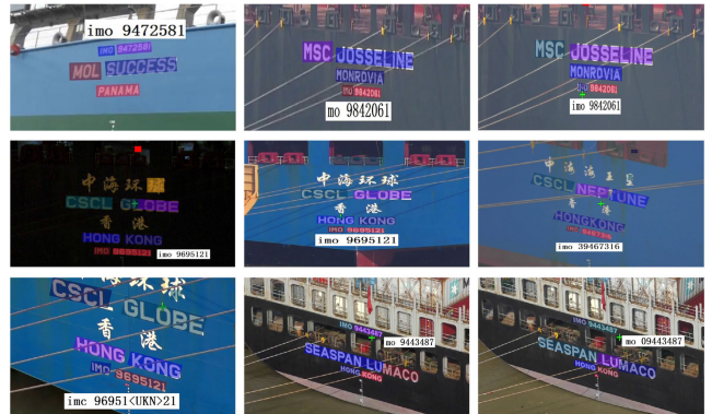
FIGURE 16. Text recognition of ship IMO region by SVTR.
