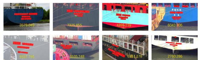
FIGURE 7. Pixel value calculation for IMO text area to be recognized in ships.
