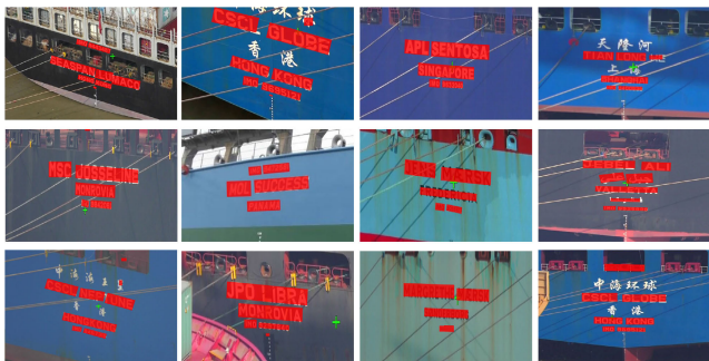
FIGURE 14. Text detection of ship IMO region by model DB_R18.
