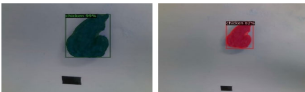
FIGURE 17. Comparison of segmented objects from the camera placed with different heights of 35 cm (left) and 55 cm (right).
