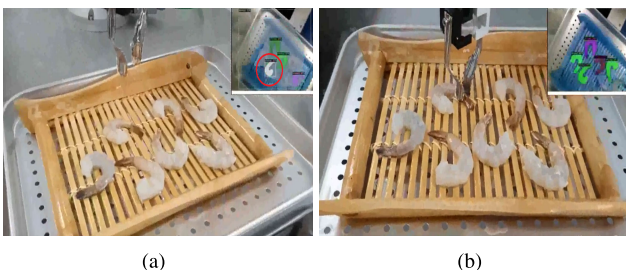
FIGURE 14. Snapshots of identifying a target shrimp (marked with a red circle) from the camera mounted on the robot hand (a) and grabbing the target shrimp (b).
