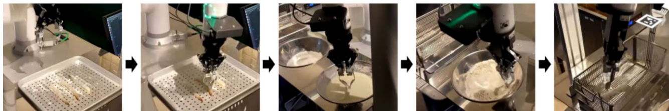
FIGURE 20. A sequence of a cooking robot system for picking up the thin areas of shrimp.
