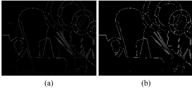
FIGURE 5. (a) Mask map of Art without binarization. (b) Mask map of Art with binarization. The binarization operation highlights the edge region of the depth image. Specifically, the mask value of the edge region is 1, otherwise the value is 0 so that the loss calculation can be performed on the edge and smooth region separately to prevent excessive smoothing of edge regions in the reconstructed SR depth image.
