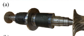
FIGURE 9. Experimental setup: (a) compressor, (b) permanent magnet rotor with compressor wheels.
