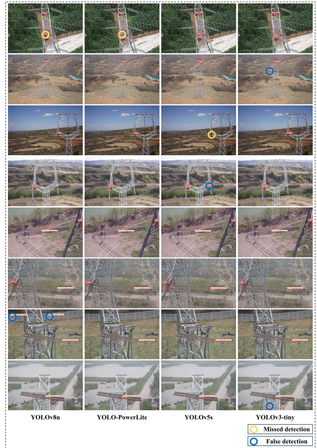
FIGURE 10. The detection results of four lightweight algorithms in abnormal target detection of transmission lines.
