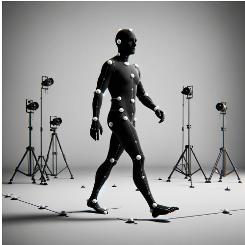
FIGURE 3. Example of collecting motion capture dataset. Multiple motion cameras are placed to capture human motions generated by an actor with tracking markers.
