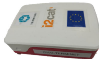
FIGURE 9. RINA-based IoT gateway.
