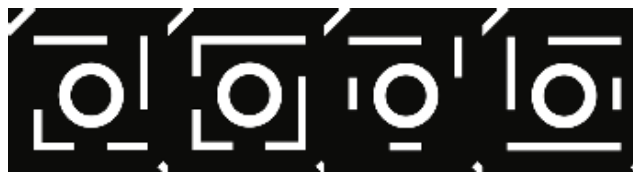
FIGURE 1. Target design: A target designed using binary coding, where each side of a square is divided into three equal parts, and the absence of a different side is indicated as "0" and the presence of a different side is indicated as "1."
