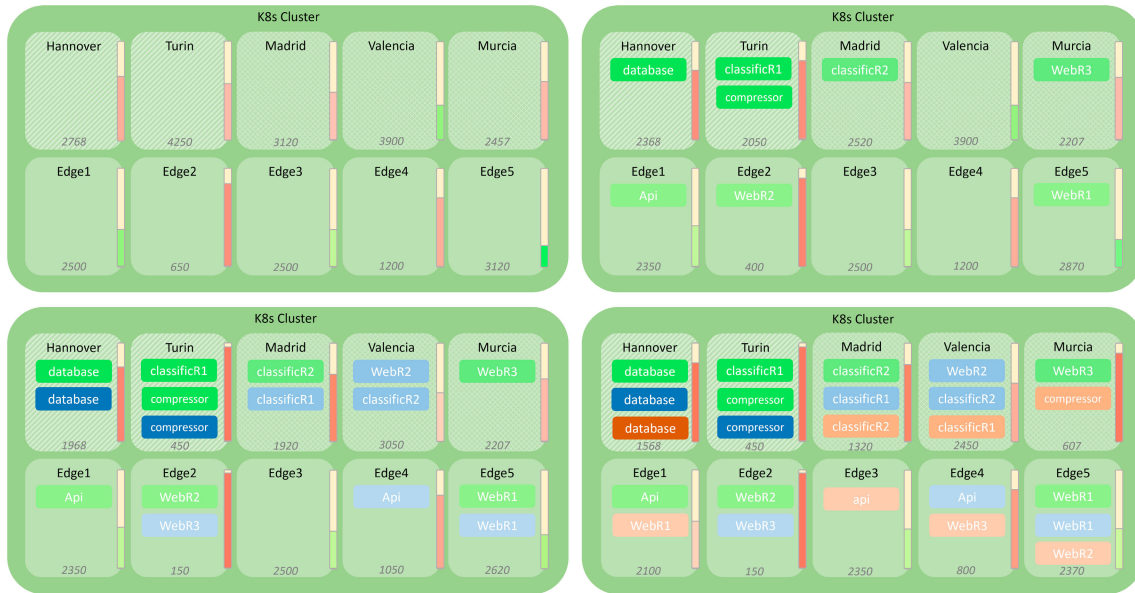
FIGURE 6. Evolution of allocating service batches to the infrastructure (from top left to bottom right).
