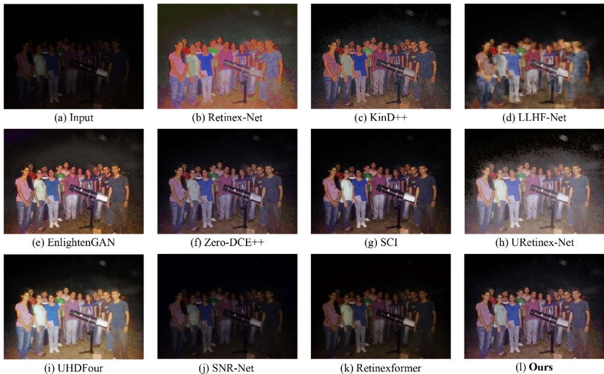
FIGURE 8. Visual comparison results with various approaches on the ExDark dataset, note that ExDark dataset does not have reference image, zooming in to get the best viewing effect.
