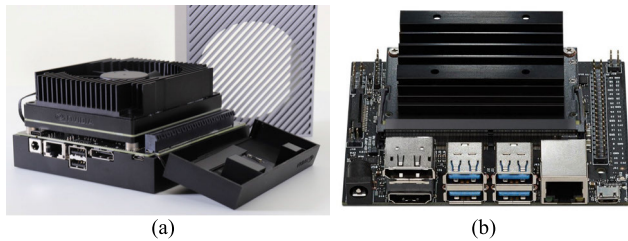
FIGURE 6. Deploying on the embedded system, (a). NVIDIA Jetson AGX Orin, and (b). Jetson Nano.
