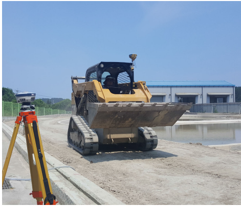
FIGURE 15. The DRB autonomous track loader with an RTK-GPS whose antenna was attached at its vertical chassis due to its convenience of installation.
