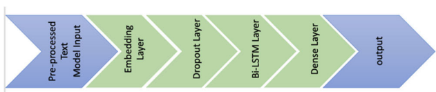
FIGURE 6. Bi-LSTM model architecture.
