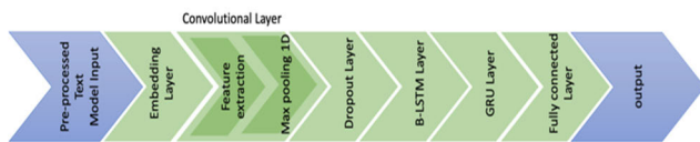
FIGURE 8. Overview of proposed model architecture.
