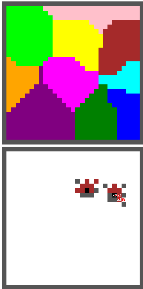
FIGURE 4. Visualization of the initial Voronoi regions for a randomly 30 \times 30 generated maze (top image). Agents within broadcast range (bottom image) have merged their Voronoi regions and exchanged information about their surroundings. Additionally, on the bottom, the red line depicts the wavefront path (x_1, x_2) from an agent (x_0) to its goal (f) within its region. The black cells represent the agents. The colored cells depict the Voronoi regions, with each color representing a different partition, whereas the darker gray cells denote obstacles.
