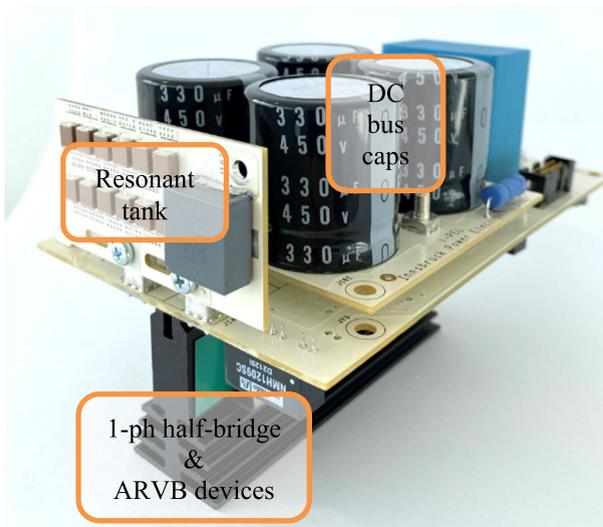
FIGURE 11. Experimental prototype of the single-phase half-bridge rectifier with an active resonant voltage balancer.
