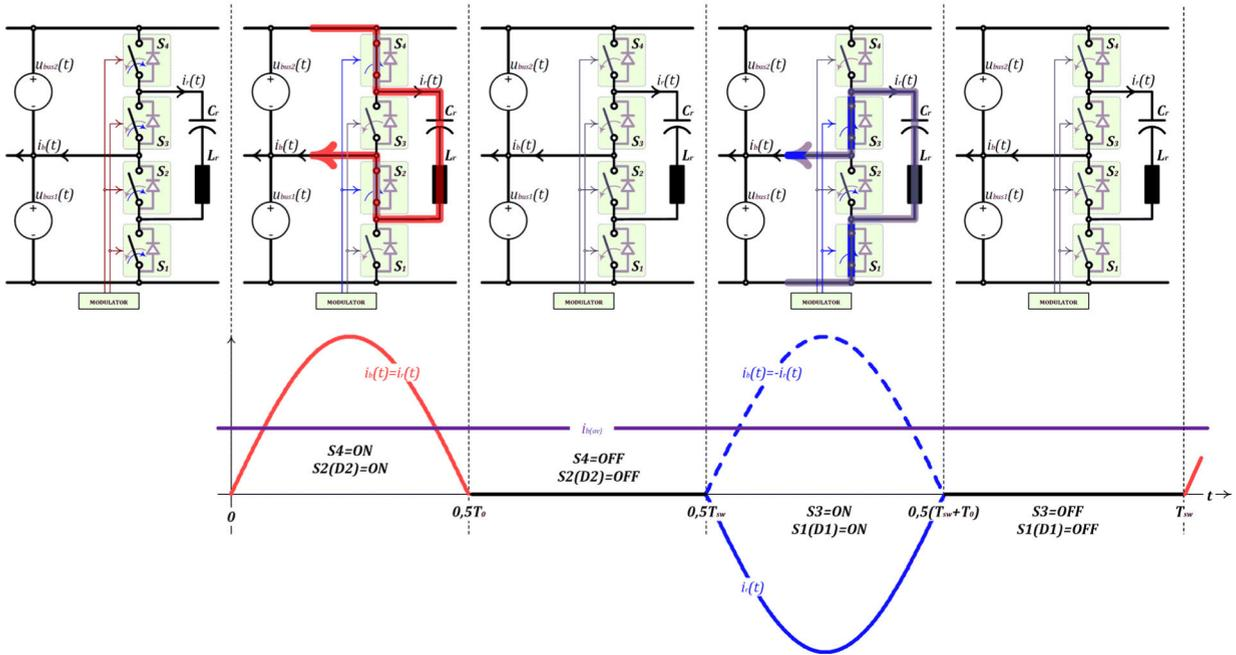
FIGURE 9. Operation of the resonant active voltage balancer.
