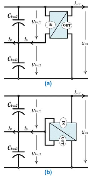
FIGURE 7. Possible arrangements of the AVB. a) Asymmetric, b) Symmetric configuration.
