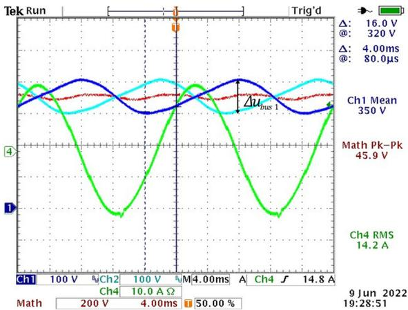
FIGURE 12. DC bus waveforms rectifier only without ARVB, Ch1 DC bus voltage upper side, Ch2 DC bus voltage lower side, Ch4 input current, Math Total DC bus voltage ripple.
