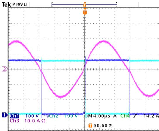
**FIGURE 14.** Experimental waveforms with ARVB, Ch1 voltage across drain source of M4, Ch2 voltage across drain source M1, Ch3 resonant current, Ch4 input current (trigger only).
