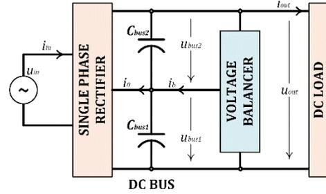
FIGURE 6. Single phase half-bridge rectifier with a voltage balancer.
