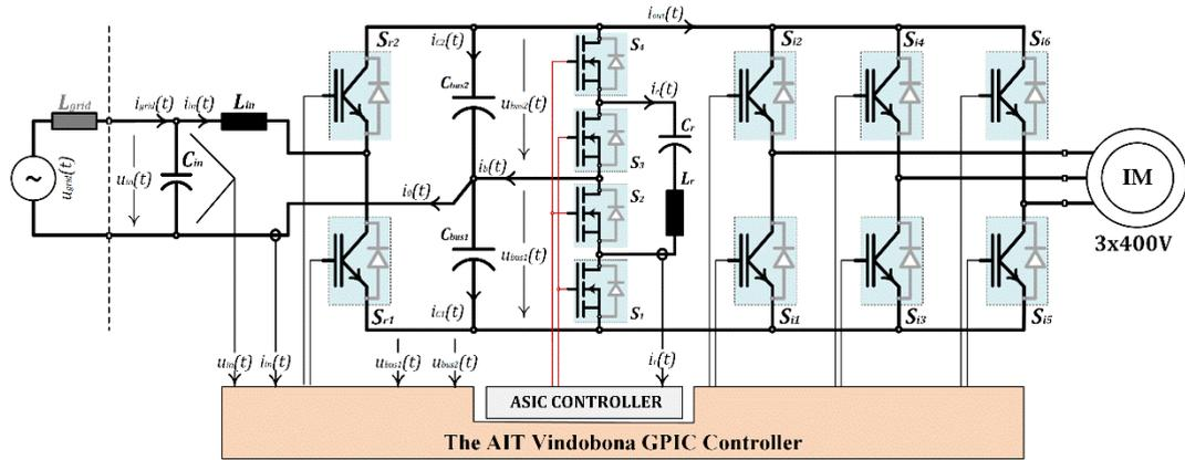
FIGURE 10. The proof-of-concept prototype circuit diagram.
