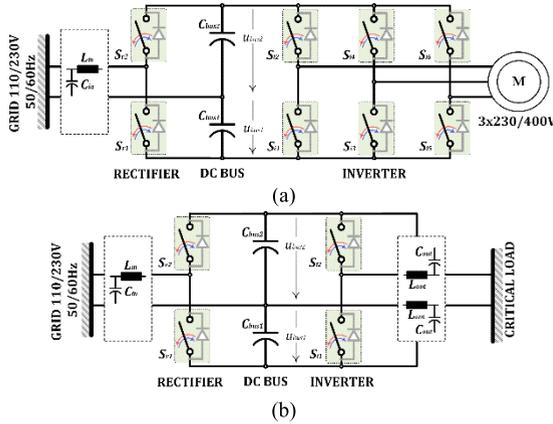
**FIGURE 1. Typical applications of single-phase half bridge rectifier. a) Single-phase to three-phase Variable Speed Drive (VSD), b) Single-phase to single-phase UPS.**
