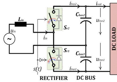
**FIGURE 2. Single-phase half-bridge rectifier.**
