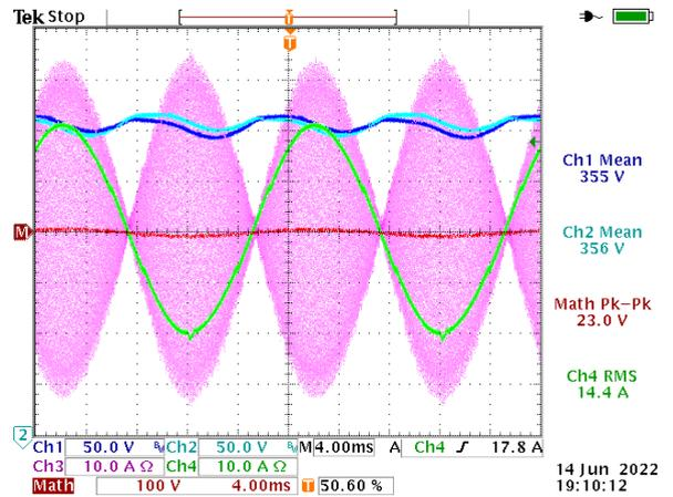
FIGURE 13. DC bus waveforms rectifier with ARVB, Ch1 DC bus voltage upper side, Ch2 DC bus voltage lower side, Ch3 resonant current, Ch4 input current, Math half DC bus voltages difference.
