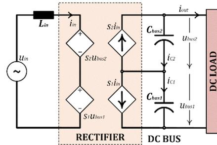
**FIGURE 3. Switching mode model of single-phase half-bridge rectifier.**
