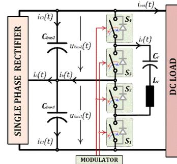
FIGURE 8. Series resonant converter as an active voltage balancer.
