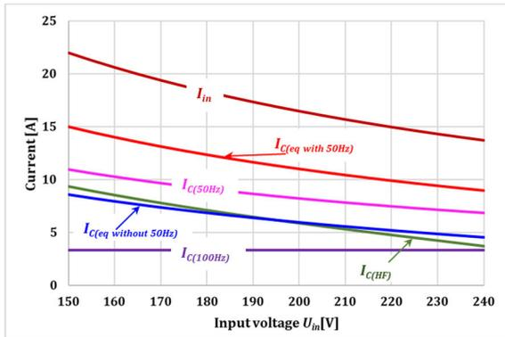
FIGURE 5. The DC bus Capacitor current stress versus input voltage. The DC bus voltage  $U_{out} = 700V$  and power  $P_{out} = 3300W$ .
