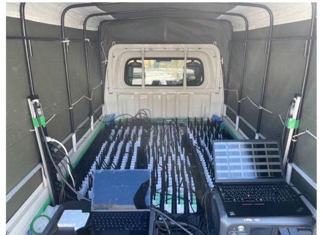
(b) Setup of an outdoor experiment at Yokosuka Research Park, Kanagawa Prefecture, Japan. Two trucks were each loaded with 500 nodes using CSS-APCMA at 920 MHz to transmit messages to a receiver antenna located at the top of a seven-storey building [19].
